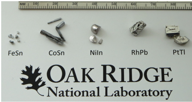
FIG. 2. A photo of the CoSn-type samples with steel scale. The pale-blue metallic luster of CoSn is evident but the pale-pink hue of NiIn does not show up well.
